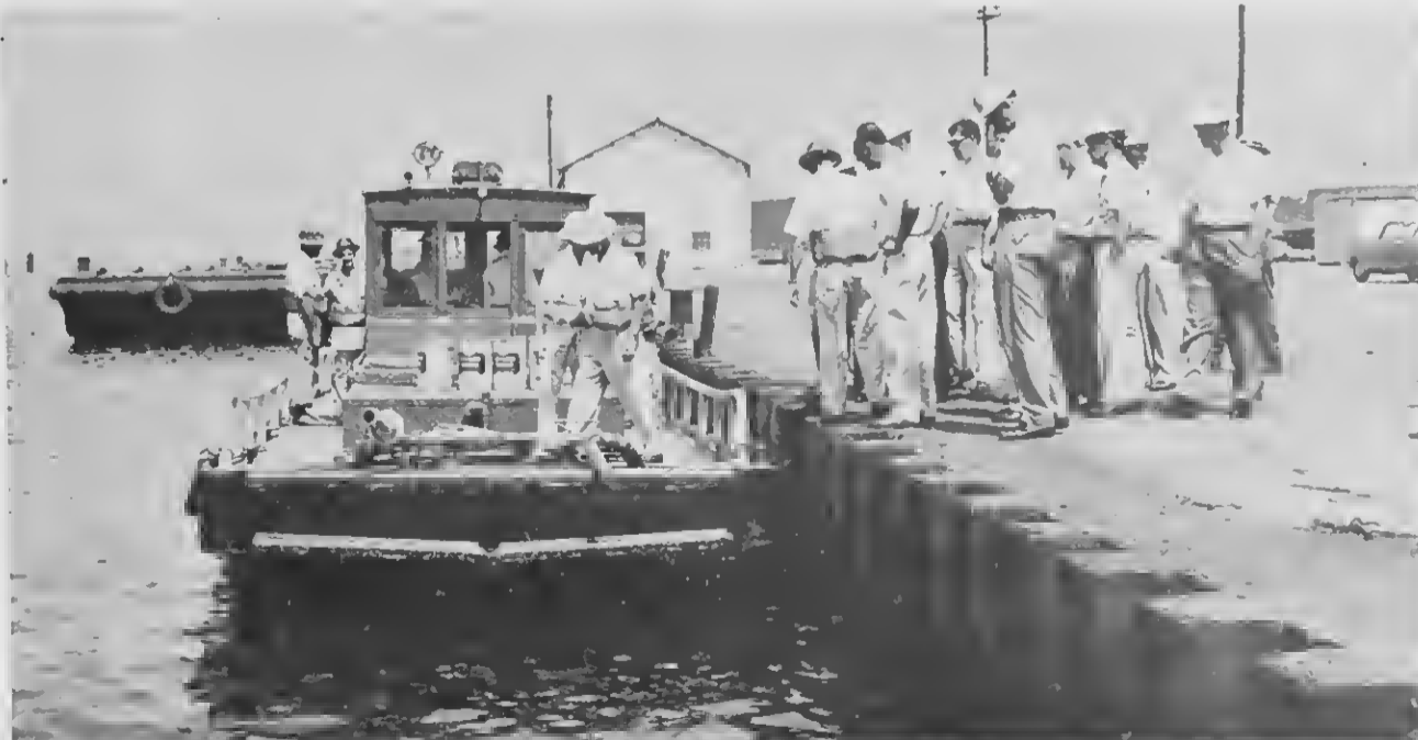
AT ACCEPTANCE trials held earlier this year, members of Management inspected the new No. 9 fire boat and boarded her for trial runs. Built entirely from salvageable materials, the fire boat was constructed at a cost less than the $18,000 fee for two gas turbines alone which were originally planned for the craft. The entire project was the brain-child of Howard Garig, head of the Floating Equipment Division of the Marine Department.
